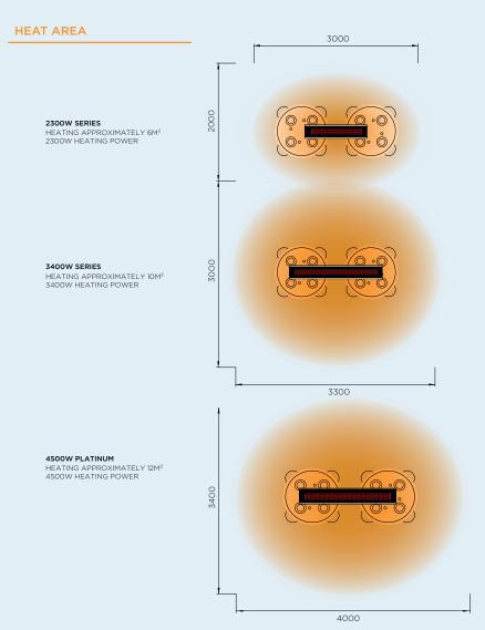
\*HEAT AREA DEPENDENT ON AMBIENT TEMPERATURE AND WIND. OPTIMUM CONDITIONS EXPERIENCED AT APPROX 15.5°C AND IN A LOW WIND COVERED ENVIRONMENT.
