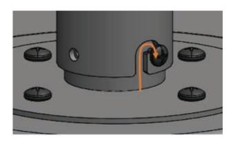
7. Fully insert additional 2 X Dome Head Screws (M4 - Length: 6mm) on both sides, and tighten all four screws, to lock heater in place.
