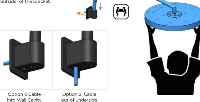
9. Fasten the Wall Mount Pole to the Wall Bracket using 1 X Round Head Hex Screw (M8 - Length: 15mm).
