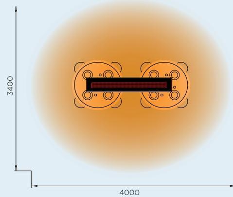
\*HEAT AREA DEPENDENT ON AMBIENT TEMPERATURE AND WIND. OPTIMUM CONDITIONS EXPERIENCED AT APPROX 15.5°C AND IN A LOW WIND COVERED ENVIRONMENT.
